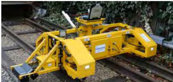
The portable Track Geometry and Conductor Rail Measurement System provides a convenient method of ascertaining many parameters simultaneously with reference to distance measurement. Small and light with a total assembled weight of approximately 100kg, each of the four parts can be lifted by two operators and used in two modes; pushed/towed by TunnelFox®.
