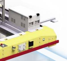
With the 3D Tunnel Scanner, TunnelFox® can capture visual and thermal images as well as 3D profile recordings all in a single recording sweep, allowing for a wide variety of analysis options. With this fox hard at work for you, you can reduce reliance on manual inspection and improve the consistency, efficiency and accuracy of tunnel fault detection.
