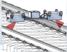
Track Geometry Measurement System
