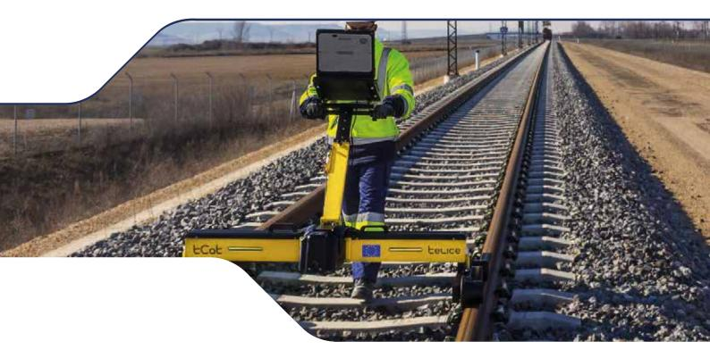
Reliable, low cost geometry measurement solution Real-time, actionable information Automatic measurement - height and stagger Foldable design, easy to transport
